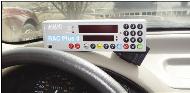
Fig. 2.8 - 'L' Bracket on Curved Dashboard
