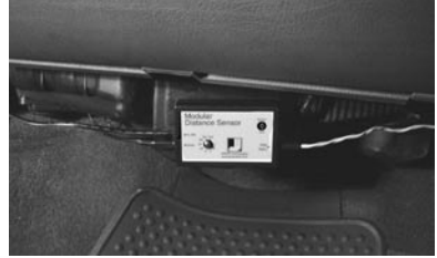
Fig. 2.1 MDS Mounted Under Dash
