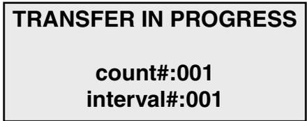
The DB-400 starts sending the data to the computer, beginning with the first interval of the first count. The screen shows the count number and interval number that is being transferred. When all of the data has been transferred, the screen returns to the Dump. Assuming the transfer is successful, you can then select EXIT to return to the Main Menu.
