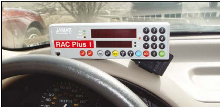
Fig. 2.9 - 'L' Bracket on Curved Dashboard
