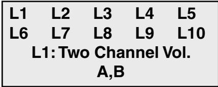
The TAB key is used to move through the layouts. A description of the currently flashing layout is displayed on the bottom two lines. Refer to Chapter 5 *Road Tube Layouts* for a more detailed description of the individual layouts.
