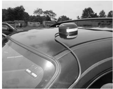
Fig. 2.20 - GPS Receiver on Roof
