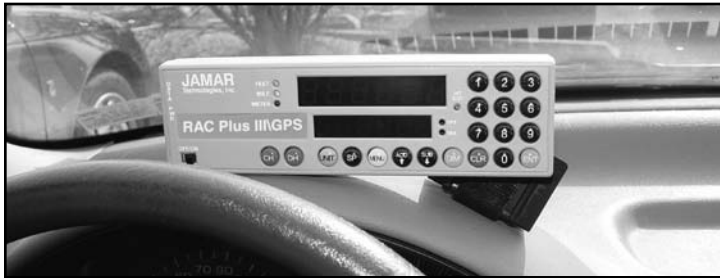
Fig. 2.19 - 'L' Bracket on Curved Dashboard
