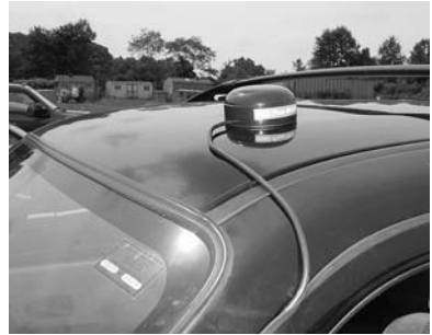
Fig. 5.2 - GPS Receiver on Roof
