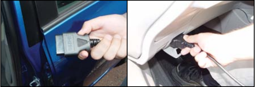
Fig. 2.1 – Plugging in to the OBD Port
