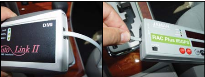
Fig. 2.2 – Connecting the OBD Sensor to the RAC Plus III
