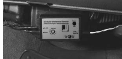
Fig. 2.3 MDS Mounted Under Dash
