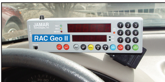
Fig. 2.2 - 'L' Bracket on Curved Dashboard
